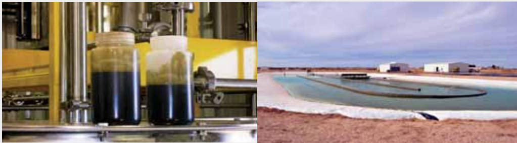
First oil from algae at the CEHMM Artesia algae plant and a quarter-acre pond with extraction facilities in the background
